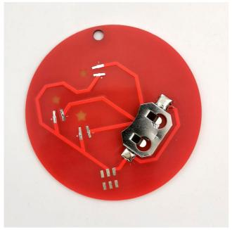
First solder one side of the battery holder to one of the two big soldering points on the PCB. The holder itself has no polarity, as long as the "+" mark faces upwards.
